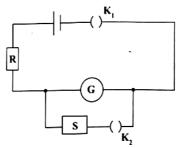
He Unplugged a resistance of 5200  $\Omega$  in R. When  $K_1$  is closed and  $K_2$  is open, the deflection observed in the galvanometer is 26 div. When  $K_2$  is also closed a resistance of 90  $\Omega$  is removed in S, the deflection becomes 13 div. The resistance of galvanometer is nearly
